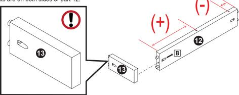
Identify the two indents on both sides of Center Drawer Rail (12), the indent with the longer distance between it and the edge of the rail must be installed toward Center Drawer Rail Support 13.
