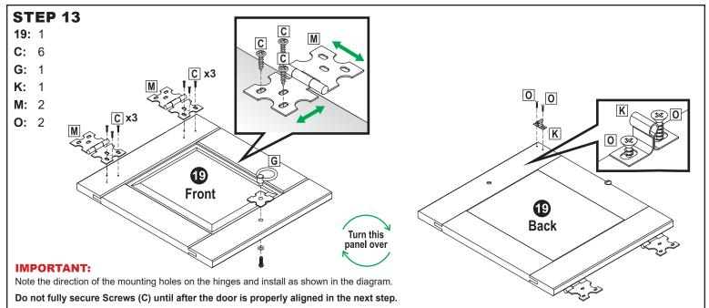
Align two Hinges (M) with the indents on the front of Right Door (19) and mostly fasten using six M3.5x14mm Pan Screws (C).
