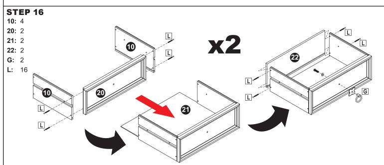
Ensuring the inside grooves align, secure two Drawer Sides (10) to Drawer Face (20) using four M3.5x30mm Flat Screws (L).
