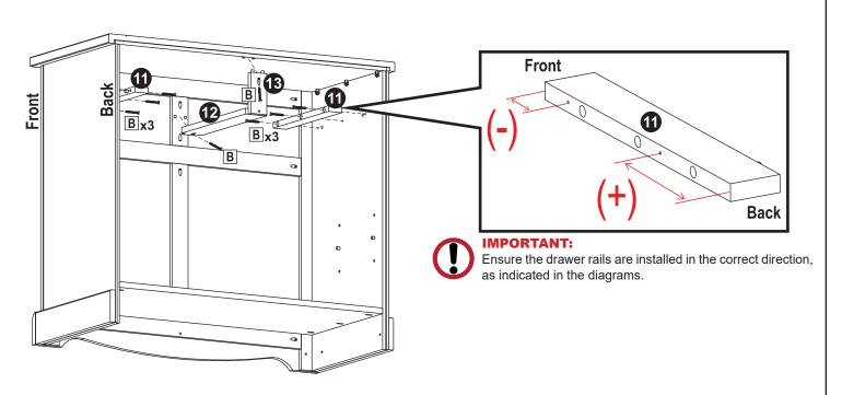
Identify the two indents on Outside Drawer Rails (11), the indent with the shortest distance between the indent and the edge of the rail must be installed toward the <u>front</u> of the cabinet.
