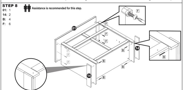
Align two Side Trim Boards (14) with the bottom of the unit, as shown. Have an assistant firmly hold the trim boards in place to ensure they remain flush with the unit while hardware is secured. From the inside of the side panels, secure each trim board using two M4.5x28mm Pan Screws (B).
