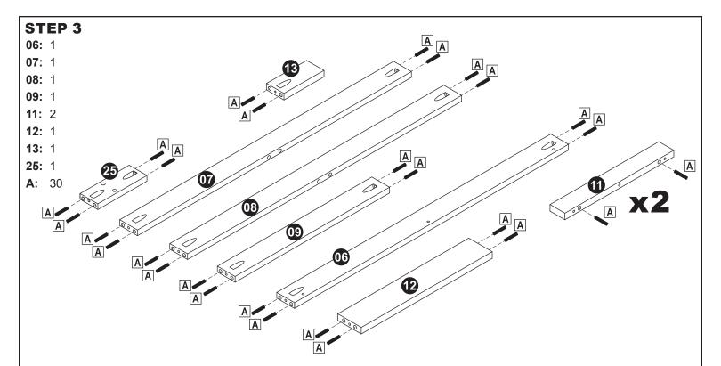
Install four Wood Dowels (A) into Bottom Frame (06), Center Face Frame (07), Top Face Frame (08), Vertical Cabinet Face Frame (09), Center Drawer Rail (12), and Vertical Drawer Face Frame (25).
