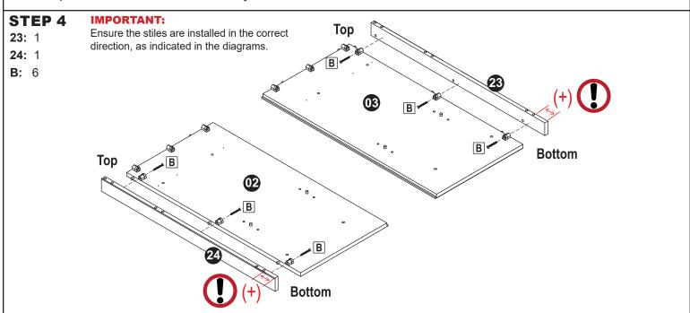
Identify the Top and Bottom of Side Panels (02,03), Left Stile (24) and Right Stile (23); the bottom of the stiles will have a larger gap between the mounting holes and the end of the panel.
