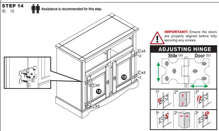
With assistance to hold the door in place, align the top hinge of the left door with the indents on the left stile. Loosely secure each hinge using three M3.5x14mm Pan Screws (K).
