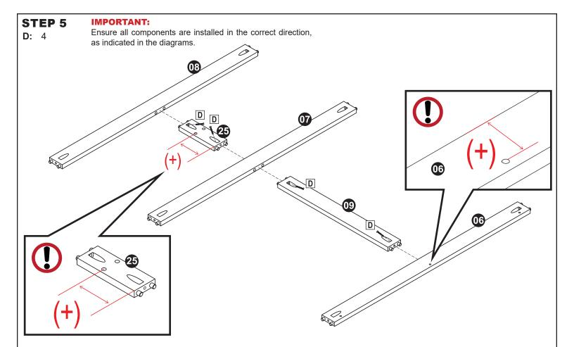
With the angled mounting holes facing upward, lay Bottom Frame (06), Center Face Frame (07), Top Face Frame (08), Vertical Cabinet Face Frame (09), and Vertical Drawer Face Frame (25), as shown.
