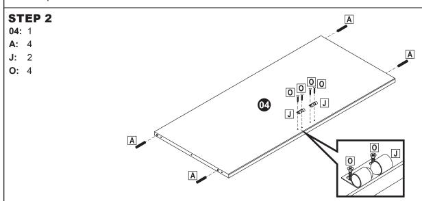
Install four Wood Dowels (A) into Bottom Panel (04), as shown.
