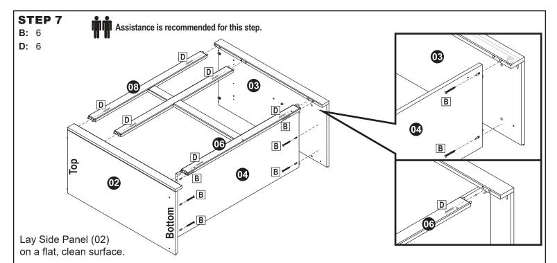
Ensuring the catches on Bottom Panel (04) face toward the top of the unit, align Bottom Panel (04) with the mounting holes on the bottom of the side panel. Then, align the assembled face frame with the mounting holes in the left stile. Secure Bottom Panel (04) using three M4.5x28mm Pan Screws (B). Then, secure the face frames using three M3.5x25mm Pan Screws (D).
