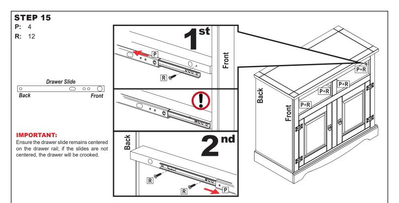
Push the front of Drawer Slide (P) backward. Align the 3rd round hole on the front of the drawer slide with the front indent on the drawer rail and secure using one M4x14mm Flat Screw (R).
