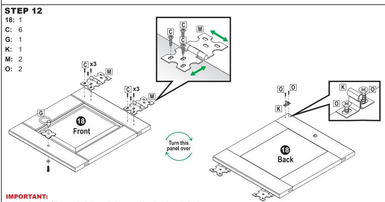
Note the direction of the mounting holes on the hinges and install as shown in the diagram.
