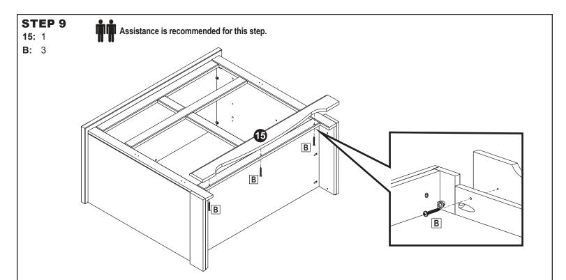
Align Front Trim Board (15) with the bottom, front of the unit. Have an assistant firmly hold the trim board in place to ensure it remains flush while hardware is secured. Secure the trim board to the bottom frame using three M4.5x28mm Pan Screws (B).
