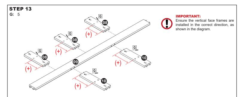
**Installation direction is very important in this step.** Identify the longer gap between the dowel mounting holes and the edge of Top Drawer Vertical Face Frames (08) and Middle Drawer Vertical Face Frames (10).
