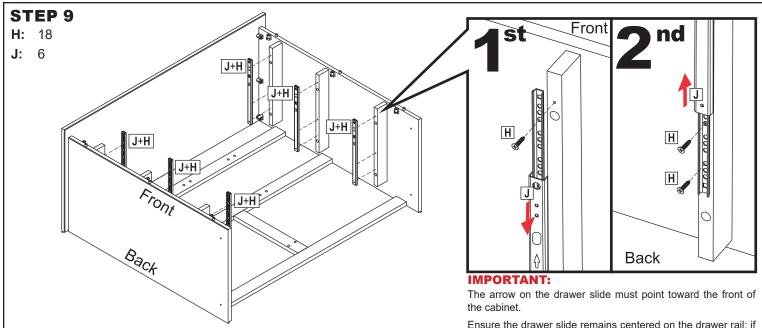
Ensure the drawer slide remains centered on the drawer rail; if the slides are not centered, the drawer will be crooked.
