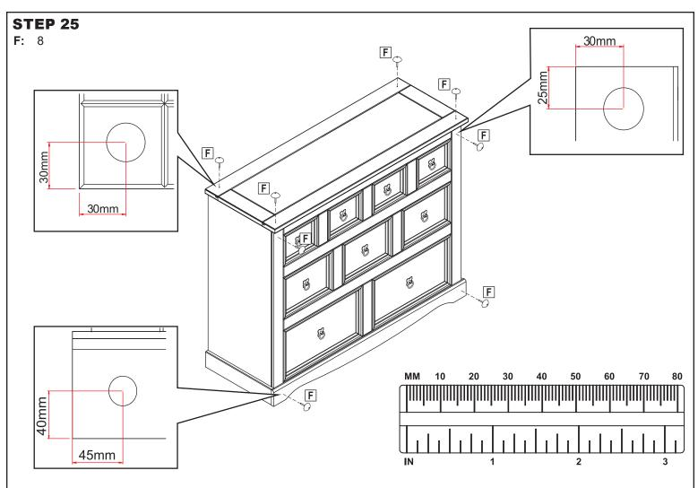
For even spacing, carefully measure and install eight Tacks (F) as indicated above.
