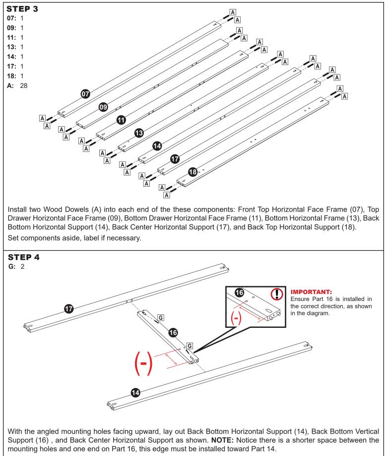
After components are aligned as shown above, secure using two M3.5x25mm Pan Screws (G).
