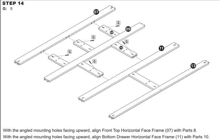
After components are aligned, secure using M3.5x25mm Pan Screws (G), as shown.
