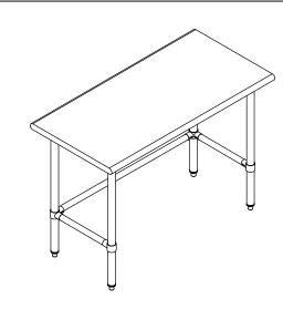
Turn over the assembled worktable, adjust the feet height to ensure proper leveling and stability, your worktable is now ready to use
