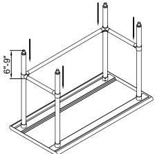
Slide the U-shape leg brace rod into the leg tube and tighten the screws after holding it at the same height. We recommend a height of 6-9 inches from the bullet foot
