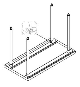
Turn the top shelf unside down onto the floor, place the carton top underneath for padding to aviod scratching, Insert four legs into the leg sockets, then partially fasten the allen screws
