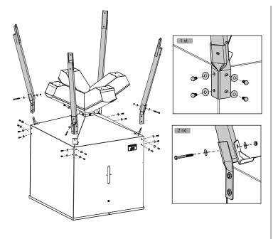
Attach upper legs to bottom of hopper using sixteen M6 x 15 mm bolts and M6 washers.
