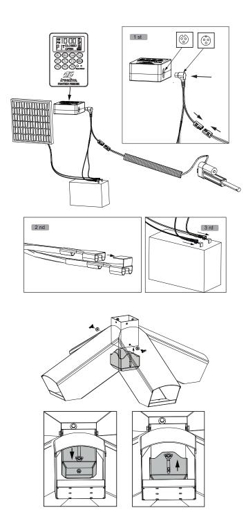
Connect wire (from actuator) to timer plug wire and insert plug into timer.
