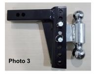
Photo 3 shows ball mount in "drop" position
