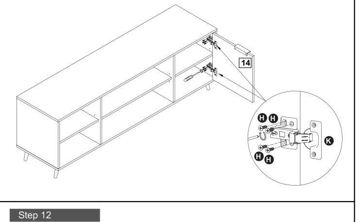
Attach left door hinge to the cabinet using (8) 3.5\*14mm Screws (Part H).
