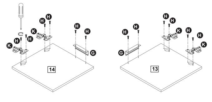
Attach (2) Handles (Part G) using (4) 3.5\*14mm Screws (Part H).
