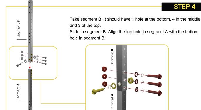
Take 4 x M8 screws and insert one Spring Washer M8 & one Flat Washer M8 on each.
