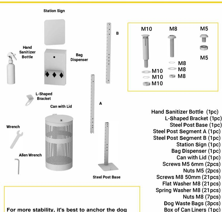
For more stability, it's best to anchor the dog waste station onto a cement pad. You will need an Air Hammer and Hammer (Not Included).
