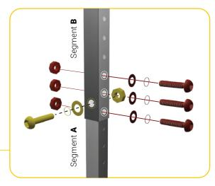
Take 4 x M8 screws and insert one Spring Washer M8 & one Flat Washer M8 on each.
