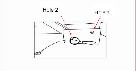
Step2: fix the pins into Hole 2.
