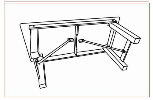
Step3.: Open the legs & fix locking pins into correct holes, then turn around the table top up.
