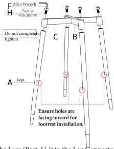
Insert the Legs (Part A) into the Leg Connectors (Part B & C) and insert (4) M8x30mm Screws. **Do not tighten screws completely at this time.**
