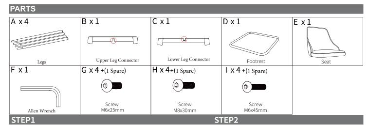
Align the cutouts in the Upper Leg Connector (Part B) and the Lower Leg Connector (Part C).
