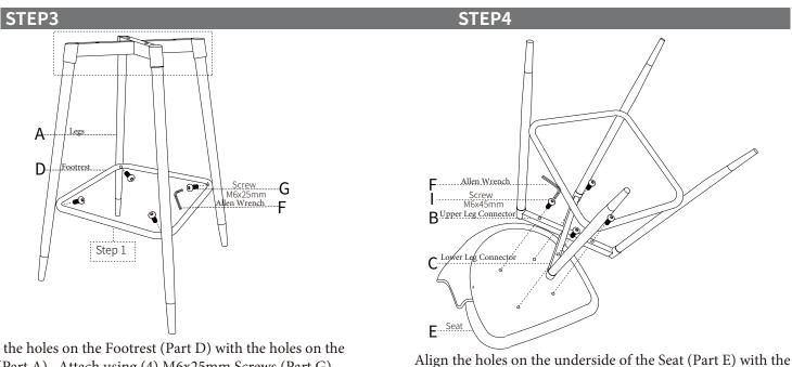
Align the holes on the Footrest (Part D) with the holes on the Legs (Part A). Attach using (4) M6x25mm Screws (Part G). Tighten using Allen Wrench (Part F). After installation of Footrest, completely tighten screws from Step 2 in the Leg Connectors.
