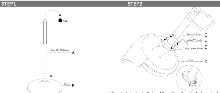
Remove the cap from the Gas Lift Cylinder and discard. Insert Gas Lift Cylinder firmly into the Base (Part B).
