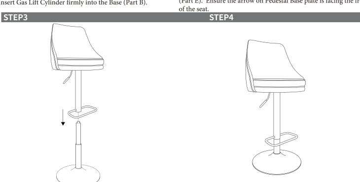
Insert the assembled Seat and Pedestal Base onto the Gas Lift Cylinder.
