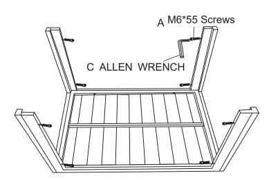
Attach (2) Wide Legs (Part E) to the Short Legs (Part D) using (8) M6\*55 Screws (Part A). Tighten using Allen Wrench (Part C)
