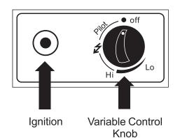
Off: the heater stops working Hi: maximum temperature position Lo: minimum temperature position
