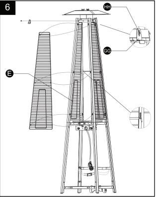
7. Assemble three side panels (G) to heater using 18pcs screw 3/16".
