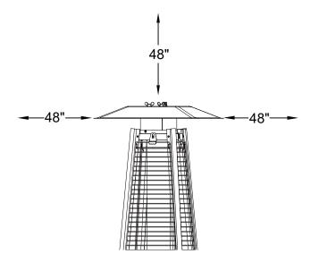
CAUTION: ANY MATERIALS OR ITEMS THAT ARE STORED ABOVE, BESIDE OR UNDER THIS HEATER WHILE IN USE WILL BE SUBJECT TO RADIANT HE AT AND COULD BE SERIOUSLY DAMAGED.
