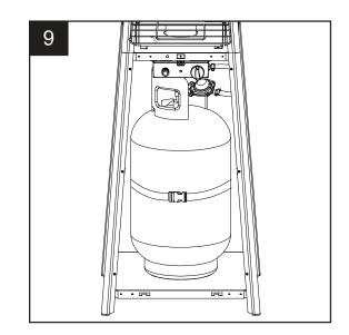
10. Turn the cylinder valve on the tank clockwise to close the propane tank. Attach the regulator (J) to the cylinder valve by turning the regulator coupling nut clockwise. Make sure it is fastened securely and tighten connections by hand only.
