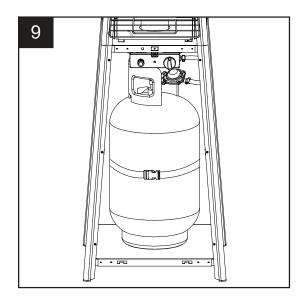
10. Turn the cylinder valve on the tank clockwise to close the propane tank. Attach the regulator (J) to the cylinder valve by turning the regulator coupling nut clockwise. Make sure it is fastened securely and tighten connections by hand only.
