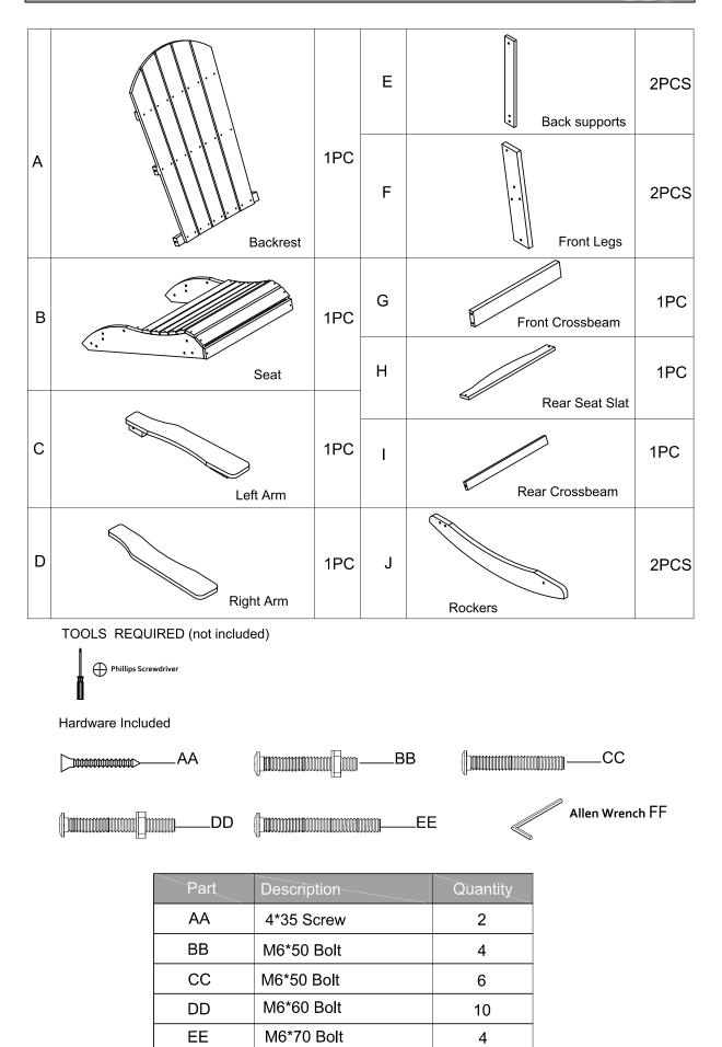
**STEP 1:** Attach the Rear Seat Slat (Part H) to the Seat (Part B) using (2) 4\*35 Screws (Part AA). Tighten using a Phillips screwdriver.
