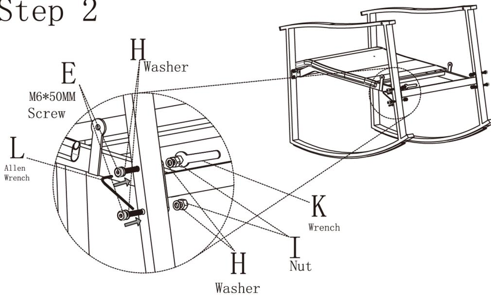
**ASSEMBLY TIPS:** Gently pull on the legs to align the holes and insert screws. Do not fully tighten until all screws, washers, and nuts are in position.
