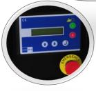
PLC Controller monitors maintenance, temp ,oil level, filtration, hours, plus remote start/stop, timed start/stop automatic restart
