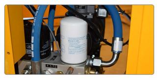
We use only genuine Mann Filters in all of our rotary screw air compressors. These filters are not exclusive to us, so after your warranty is up, you will still be able to find these filters. Mann Filters are made with superior quality and provide optimum protection against harmful elements.
