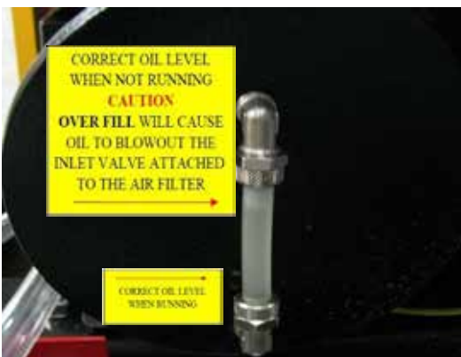
Figure 6: Sight Tube for Lubricating Oil
