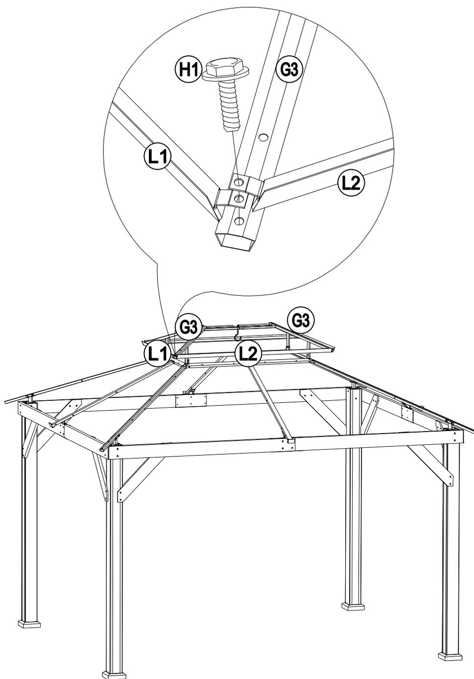
Lay Small Roof Short Roof Panel (M1) and Small Roof Long Roof Panel(M2) on the small top, Lock the Small Roof Short Roof Panel(M1), the Small Roof Long Roof Panel(M2) and Small Roof Rafter(G3) by using bolt(H1), Lock the Small Roof Short Roof Panel(M1) and the small top short side lower baffle pipe (L1), Lock the Small Roof Long Roof Panel(M2) and the Small Roof Long Panel Flashing(L2) by using Wrench(HW1)
