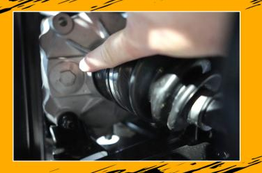
You will need an 18" extension with 17mm 6-sided socket. Remove Drain Plug.
