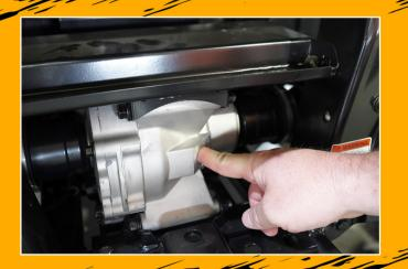
Check the oil level by placing your finger inside the drain plug.
