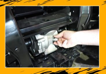
Using a 17mm 6-sided socket (do not use 12-sided socket) loosen the Drain Plug.
