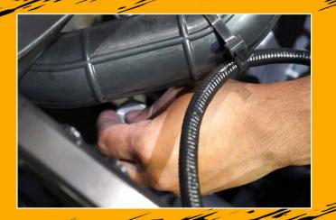
The Fill Port will hold 2.3 qts. of oil. Use the levels on the Dip Stick to determine how much oil to add.
