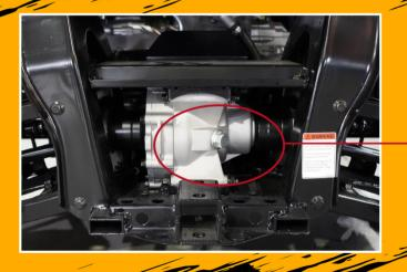
The Rear Differential drain plug is located here.
