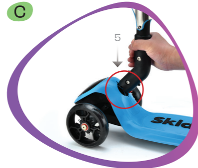
Press Red Push Button (1), Direct the Convex (3) to the Localization gap (5), Insert the Handlebar (2) in Scooter Hole (4), Until you hear the "click" sound to ensure Handlebar (2) securely locked in Scooter Body.
