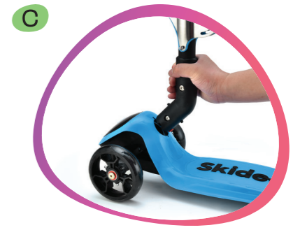
Press the Red Push Button (1) and Pull the Handlebar (2) 45 degrees upward, as shown in Figure B&C.
