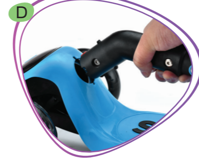
Rotate the handlebar (2) 90 degrees, Press red push button (1), Direct the Convex (3) to the Localization gap (5), insert the Handlebar (2) in Scooter hole (4), as shown in figure D&E. Until you hear the "click" sound to ensure handlebar (2) securely locked in the scooter body.
