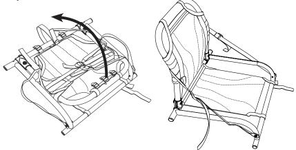
• On the bottom of the seat, wrap the wings of the seat around the seat frame and securely tighten the straps.
