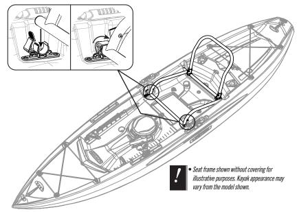
• Secure the long, center strap on the underside of the seat cover to the tie-off bracket on the hull. This will prevent the seat from sinking in the event that the seat becomes seperated from the hull in the water.
