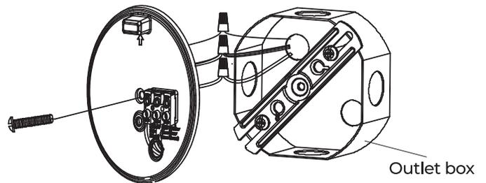
5. Attached the light fixture to the back plate using the center mounting screw:
