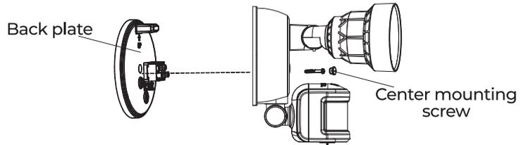
3. Connect the source wires from the outlet box with the wires of the back plate using wire nuts as follows:
