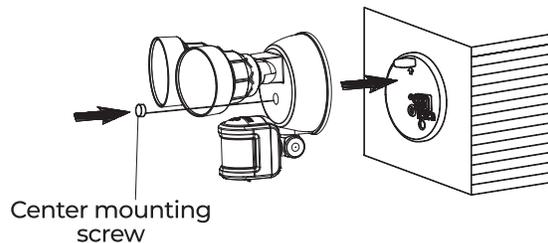
6. Using silicone caulking compound, caulk completely around where the light fixture meets the wall surface to prevent water from seeping into the outlet box.
