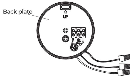
4. Place the back plate against the outlet box, insert the mounting bracket screw through the back plate hole, thread mounting bracket screw into the center hole of the mounting bar. Tighten the mounting bracket screw securely.
