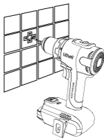
Drilling in tiles without skidding
