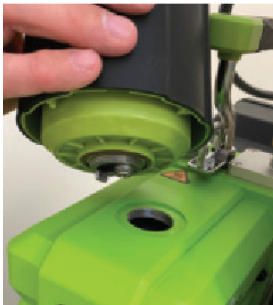
FIGURE 7: Demister removed, showing oil opening
