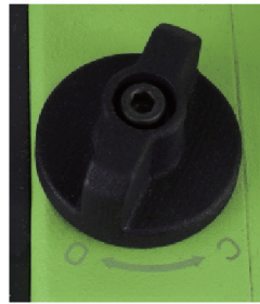
FIGURE 6: Gas ballast shown in "open" position
