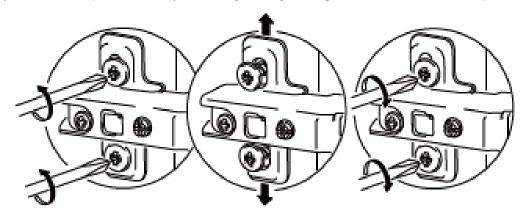
Adjust the door front and back with the left screw in the horizontal position.
