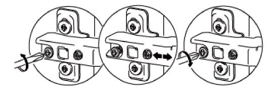
Adjust the door left and right with the right screw in the horizontal position.
