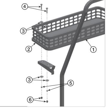
NOTE: A Phillips Screwdriver and a 13mm wrench will be a required to tighten the Screws and Hex Nuts.
