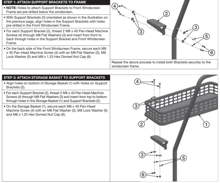
NOTE: A Phillips Screwdriver and a 13mm wrench will be a required to tighten the Screws and Hex Nuts.
