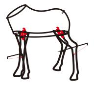
The overlapping ring between the leg and the body are fixed with tie straps, and the supporting rod is inserted into the round tube of the leg.
