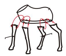
The 4-legged iron hook latch is inserted into the corresponding 2 round tubes at the bottom of the deer's body.
