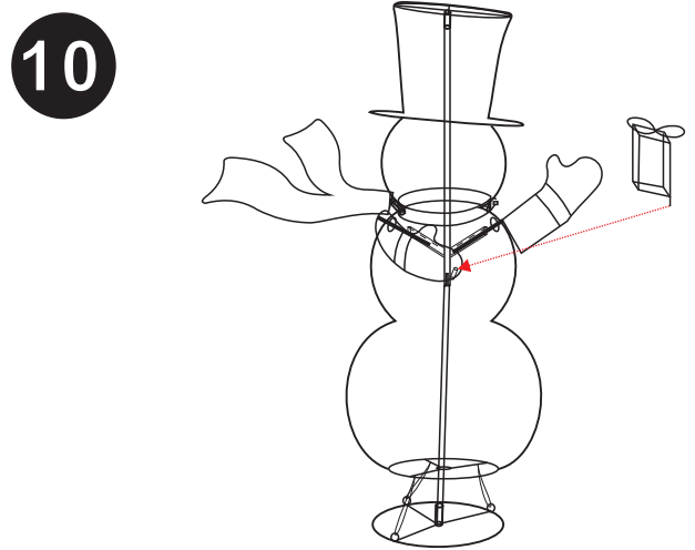
The insert pin at the bottom of the gift box is inserted into the round tube in the snowman's palm.
