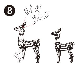
The antler latch of the male deer is inserted into the round tube corresponding to the top of the deer head.
