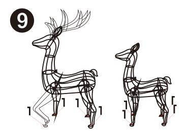
Four ground nails are inserted into the base of the deer's foot to secure it.
