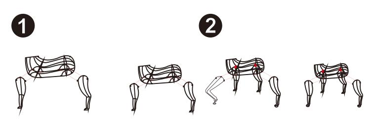
The right leg iron frame bolt is inserted into the round tube on the right side of the body.
