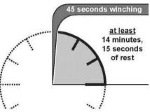
failure. Do not attempt to pull full rated load for more than 20 seconds. Release Power-In switch immediately when winch drum/rope stops. Allow winch to cool and change rigging as needed before continuing pull.
