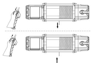
14. If using the wireless remote, press the red button for the LED to light up. Press IN or OUT to operate winch. To turn off the remote, press the red button until the LED turns off. The remote will automatically power off in 5 minutes if it is not used.
