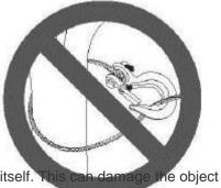
Do not wrap the rope around the object and hook onto the rope itself. This can damage the object being pulled, and kink or fray the rope.
