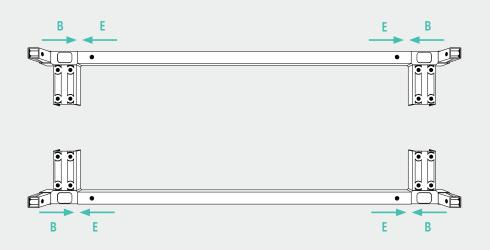
Connect the Base Width Supports (F) to the Base Connectors (B) as seen below.
