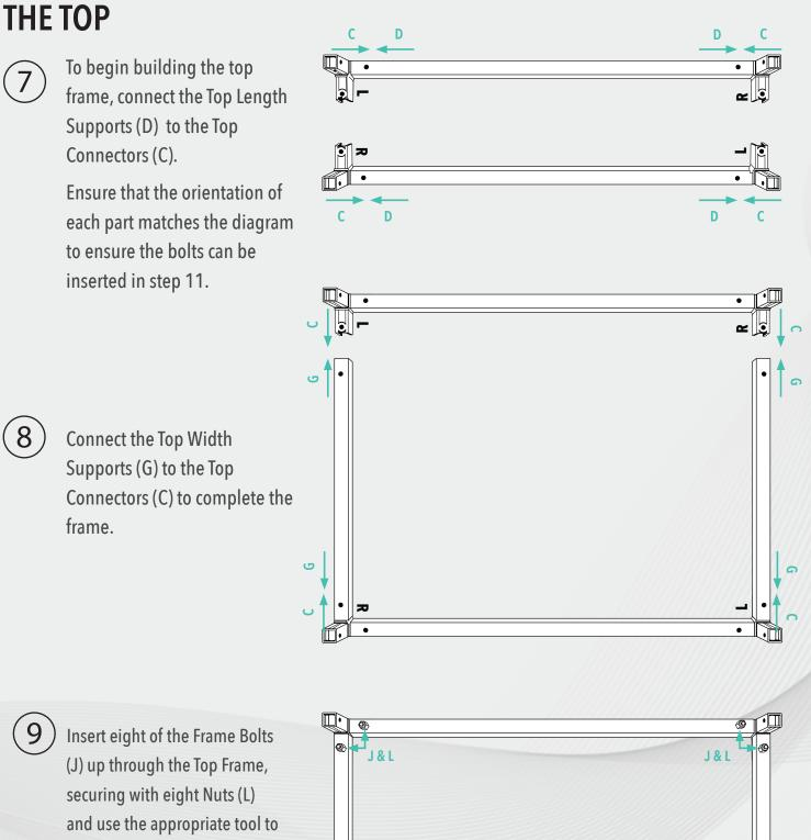
The Top Frame is now complete and ready to be connected to the main frame.
