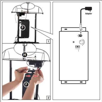
Now, plug the Adapter into the input receiving jack marked "DC 5.9V" on the Function Control Box. Note: Do not plug the Adapter into power outlet until item assembly is completed.
