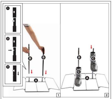
NOTE: The longer end of the (A) Base goes towards the front. First, assemble x2 of the (B) Lower Support Poles to the (A) Base as shown and secure by aligning the quick-connect push buttons into the pre-drilled holes.
