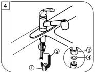
Install Weights(1) onto spray hose (2).Connect hose to outlet tube(3) and tighten. Do not overtighten.
