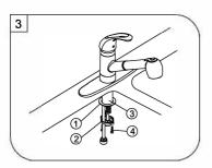
Assemble Washer(1),and thread Mounting Nut(2) onto Shank(3) from underside of sink.Handtighten.Secure Locking Screws(4) on Mounting Nut(2) and tighten Locking Screws(4)
