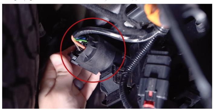
**NOTE:** If you do not have a 7-pin trailer connector or the provided plug does not fit, you may proceed with the installation using the included T-tap wire with an amp connector. Simply tap into a 12-volt power source, and plug the amp connector into the HitchMount wire harness.
