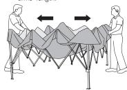
Grasp the top and bottom of the truss on opposite sides. Slightly lift canopy up and PUSH hands together while stepping backwards until canopy is fully opened.
