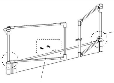
**Second**: Install gate stopper (12) with screws (11) on the inner side of the board to prevent the gate from swinging inward
