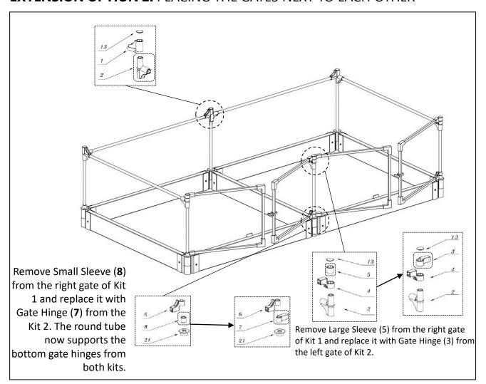
**NOTE**: When installing an extension kit on the left side of the Kit 1, instead of on the right side as shown in the diagram, Large Sleeve (5) from the right gate of Kit 1 will be replaced with <u>Gate Hinge (4) from the right gate of Kit 2.</u>
