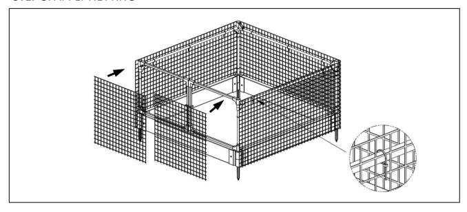
Apply the netting to both the vertical and horizontal tubes of the gates and main frame using zip ties. Attach the top of the netting flush with the upper tubes so the netting hangs over your raised bed.
