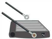
1. Lower tailgate and remove one side of the attached cables. Leave the other side attached to support the tailgate during installation.
