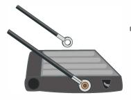
1. Lower tailgate and remove one side of the attached cables. Leave the other side attached to support the tailgate during installation.
