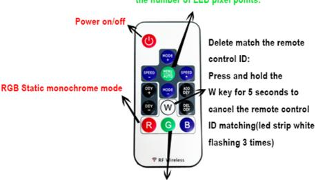
Remote control ID match: long press "G" key 5 seconds, remote control one to one match (led strip greenflash 3 times)
