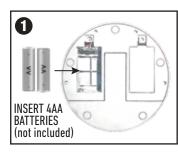
Using a small screwdriver, remove the battery compartment door. Insert 2 AA batteries. Tighten the screw to secure the cover. Repeat for the other battery compartment (total of 4 AA batteries).
