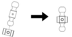
a. Align the hitch ball hole with the center of the bracket hole
