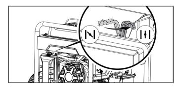
9. Press and hold the ignition switch in the "START" position for up to 5 seconds or until started.
