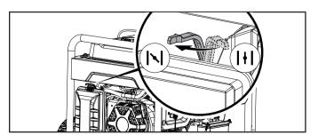
7. Press the ignition switch to the "START" position for 2-3 seconds.
