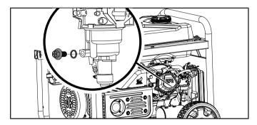
5c. When gasoline stops flowing from the carburetor, replace and tighten the carburetor drain bolt and be sure to properly dispose of the drained gasoline according to local regulations or guidelines.
