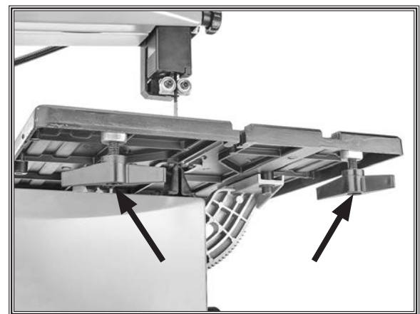
Figure 14. M6-1 x 16 fence rail knobs installed.
