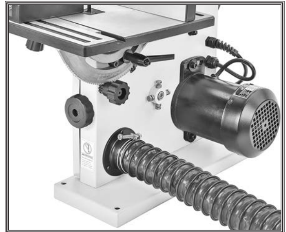
Figure 22. 2" dust host attached to dust port.
