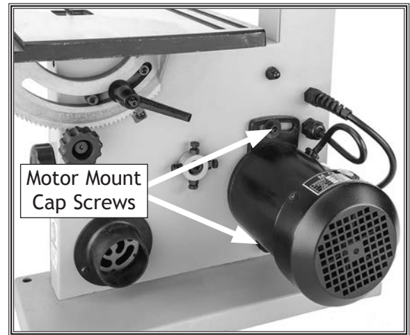
Figure 45. Location of motor mount cap screws used for adjusting belt tension.
