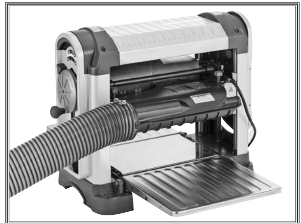
Figure 11. Dust hose connected to dust port.
