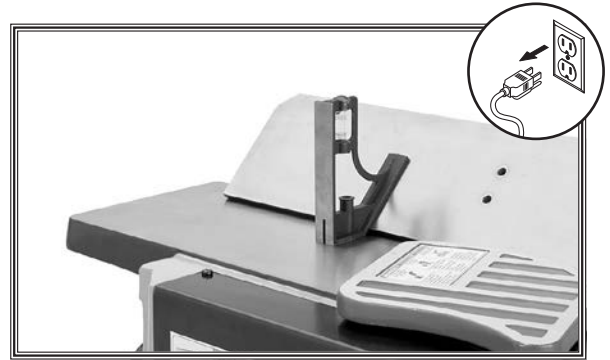
Figure 49. Example of checking 45° outward fence angle.
