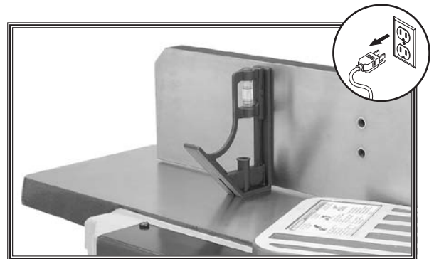
Figure 47. Example of checking 90° fence angle with combination square.
