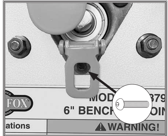
Figure 16. Installing cutterhead lock on Model W1879.
