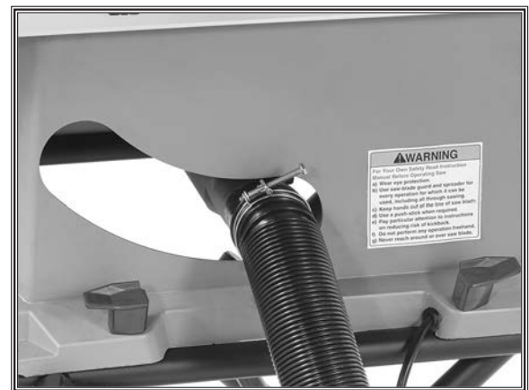
Figure 15. Dust port connected to dust collection system.
