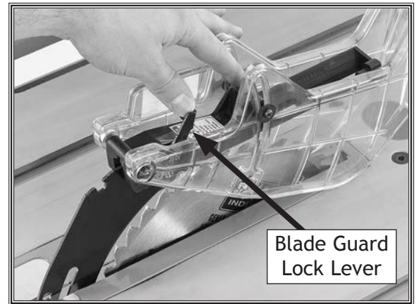
Figure 28. Placing blade guard on spreader/riving knife.
