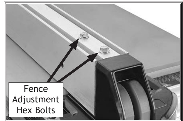
Figure 73. Location of hex nuts to adjust fence parallelism.
