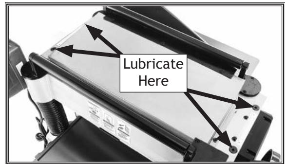
Figure 37. Lubrication locations for feed roller bushings.
