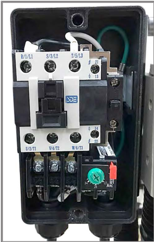
Figure 64. W1864 magnetic switch with cover removed.
